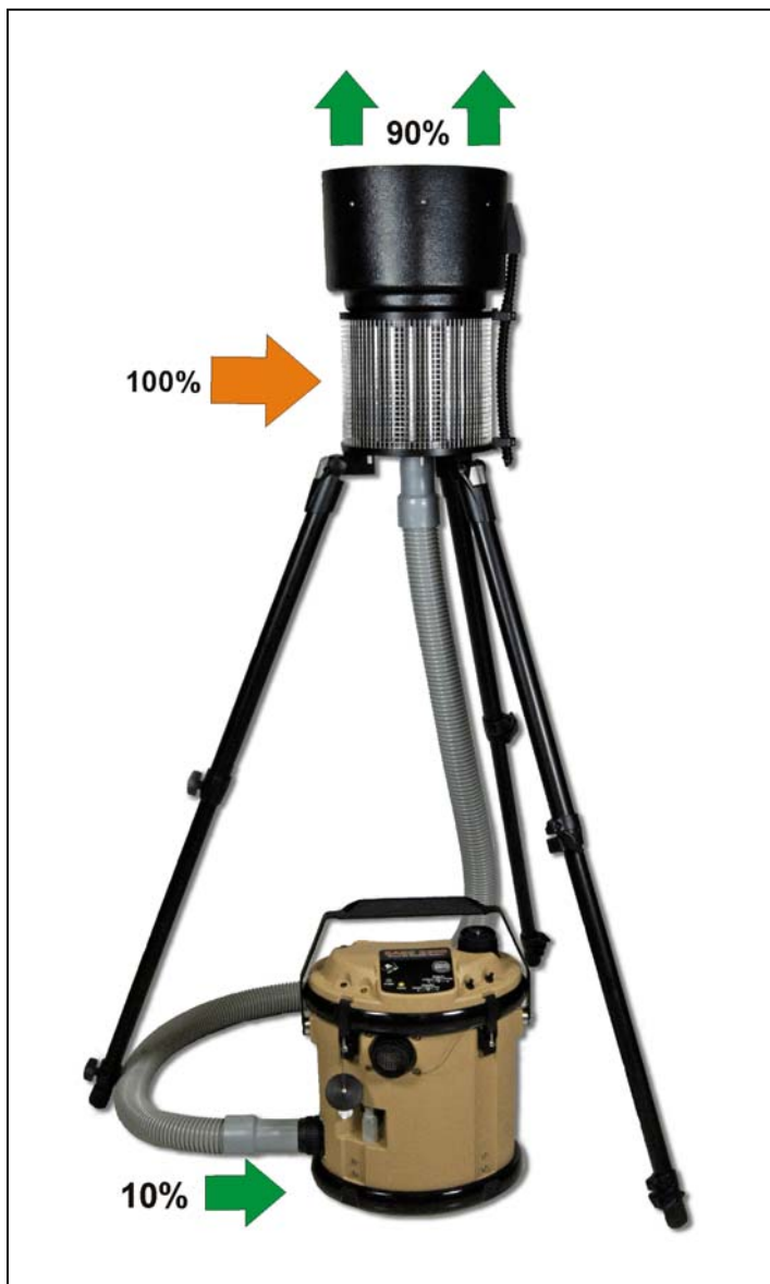
Figure 3: Airflow patterns for the SASS 4000 Concentrator.
